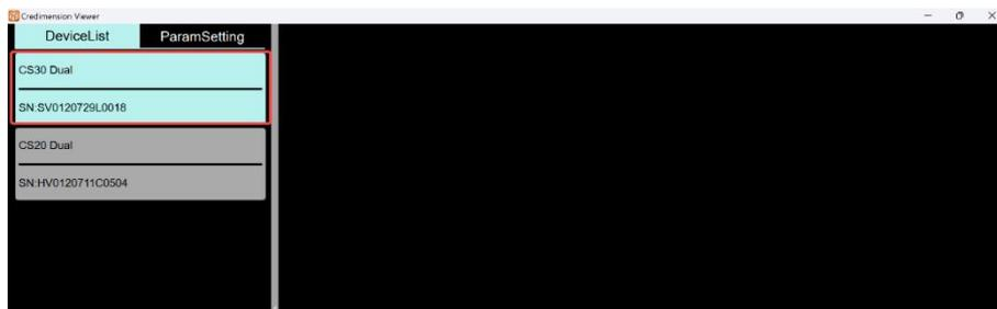
Once a device is selected, click "Param Setting" to display information about the current device, including device name, device SN, SDK version, firmware version, etc. At the same time, you can turn the current device on or off. As shown below:
