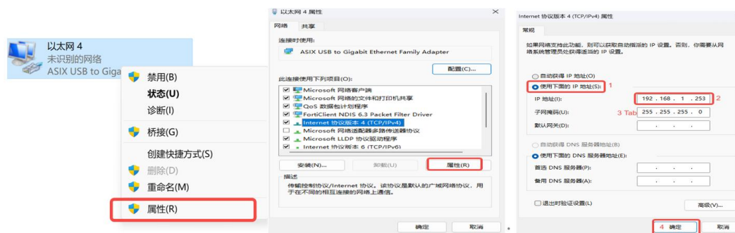
Figure 4-2.CS40 Configuring IP Steps 1, 2, and 3
